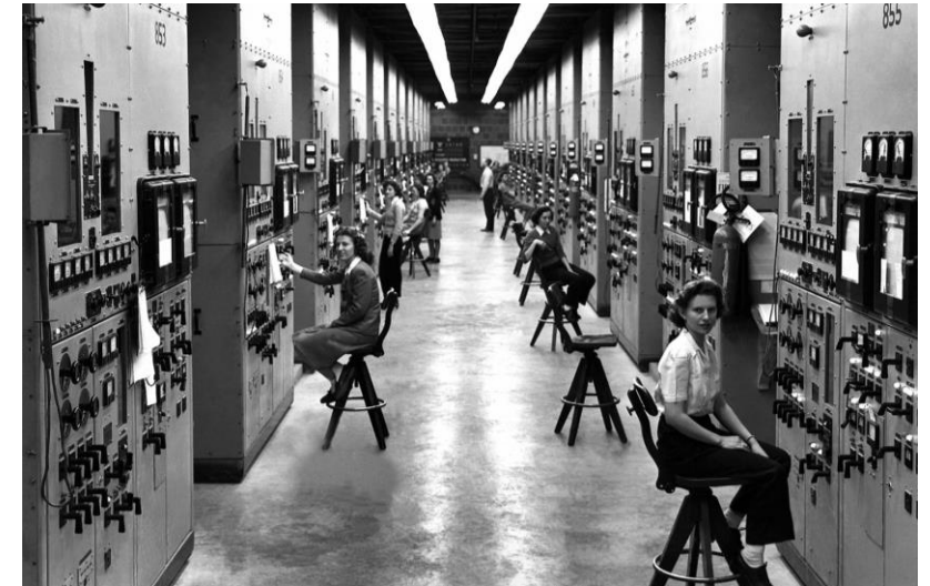
“The Calutron Girls” operating the Calutron apparatus that produced the weapons-grade uranium in Oakridge, Tennessee.
